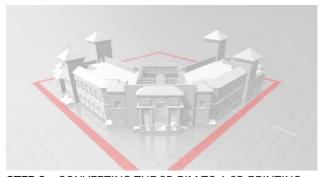
**STEP 3.** CONVERTING THE 3D BIM TO A 3D PRINTING MODELS TO ANALIZE AND DETERMINE THE ENERGY ZONES, AND ENERGY LOSES LOCATIONS.
